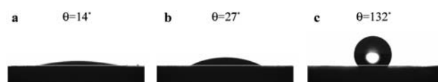
Fig. 2 Images of water droplets on pellet-type (a) HY(200), (b) FS1-Y(200) and (c) FS4-Y(200).
